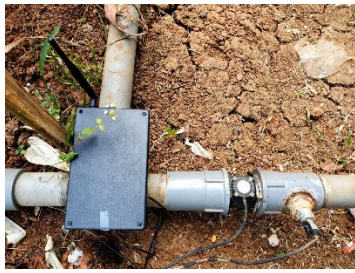
Gbr 8. Implementasi Transmitter Sensor Air
