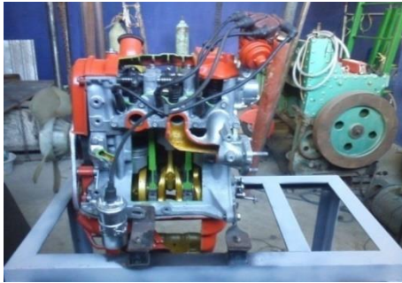
Gambar 6. Hasil Engine Cutting
