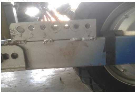
Gambar 6. Lubang Pengaturan Shock Absorber
