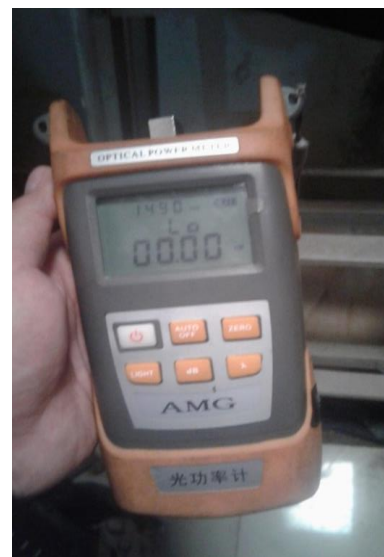
Gambar. 4 OPM (Optical Power Mater).
