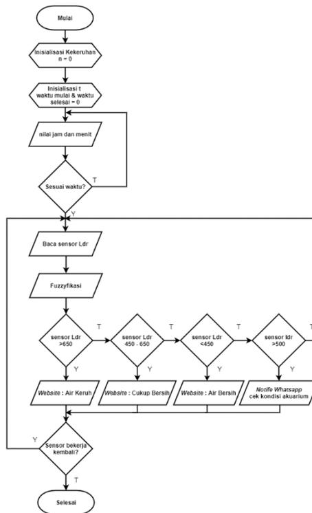
Gambar 4 Flowchart Sensor Ldr
