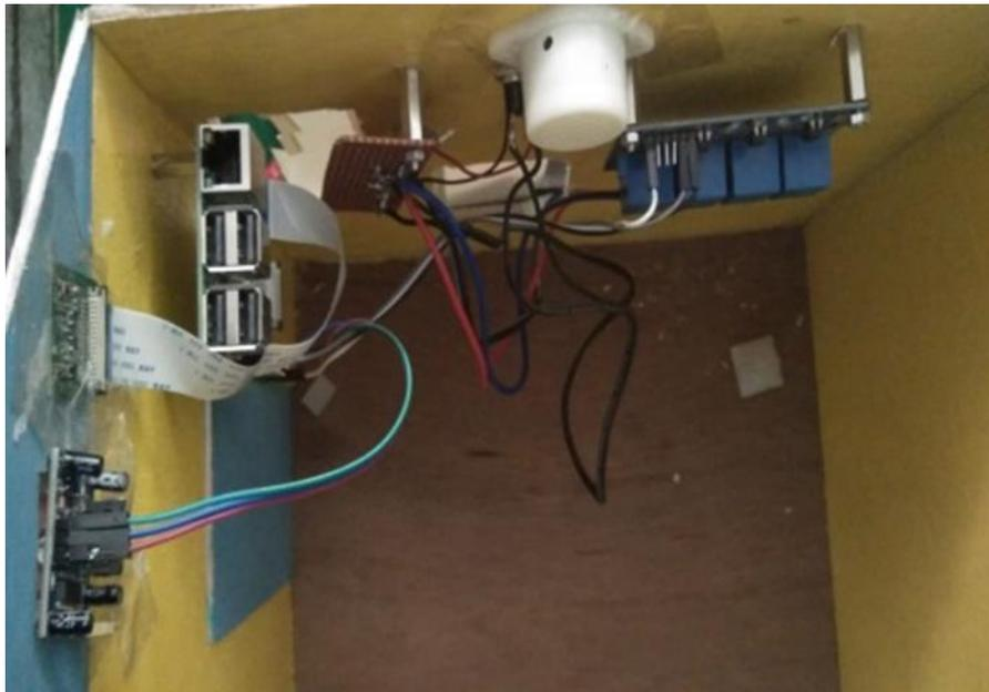
Gambar 6. Raspberry Pi Type B, Relay, dan Buzzer.
