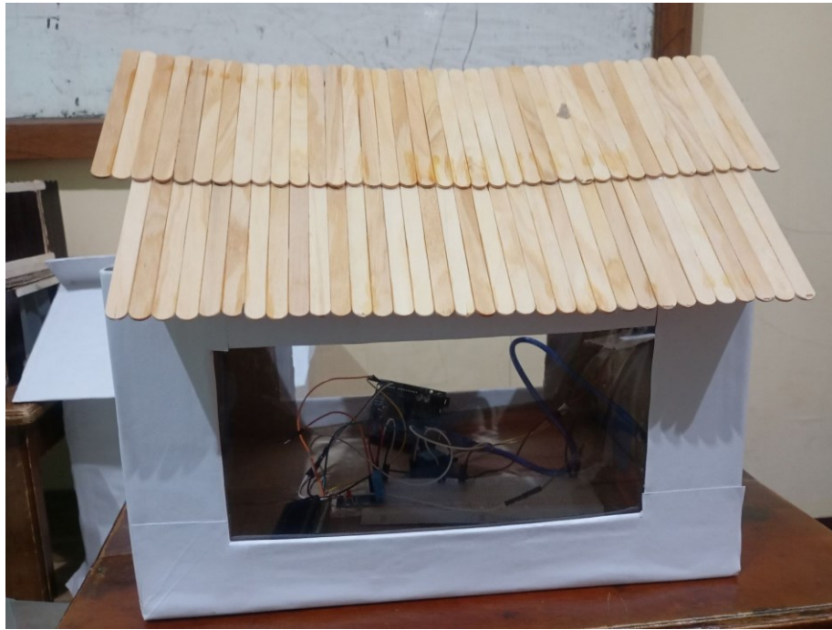
Gambar 6. Prototype Sistem Monitoring Suhu Kandang Ayam Otomatis
